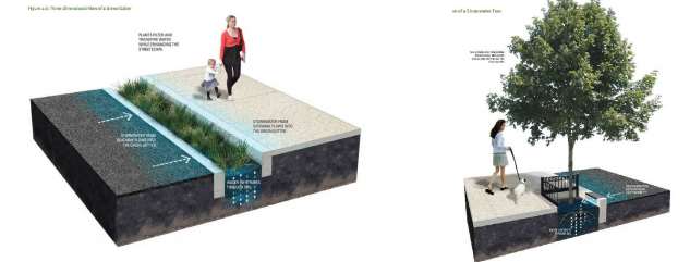
Figure 2.1: Three Dimensional View of a Stormwater Bump-out
