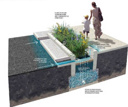
Figure 2.2: Three Dimensional View of a Stormwater Planter
