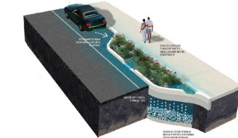
Mid-block Stormwater Bump-out
