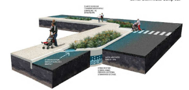
Corner Stormwater Bump-out
